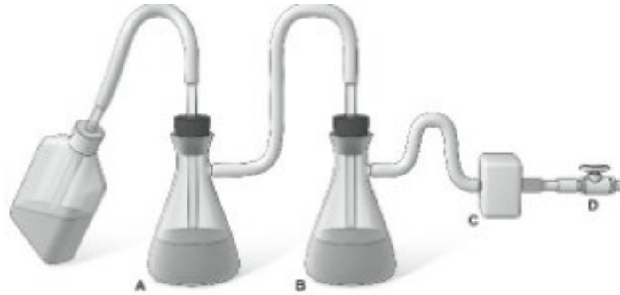
Figure 8: To collect liquid biohazardous waste, aspirate liquid into a flask containing appropriate disinfectant (A) connected to second overflow collection flask (B) and separated from vacuum system (D) by an in-line filter (C). All biohazardous waste must be properly neutralized before disposal. Source: Biosafety in Microbiological and Biomedical Laboratories, 6 th Edition
