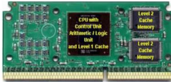
A microprocessor with its CPU and memory
