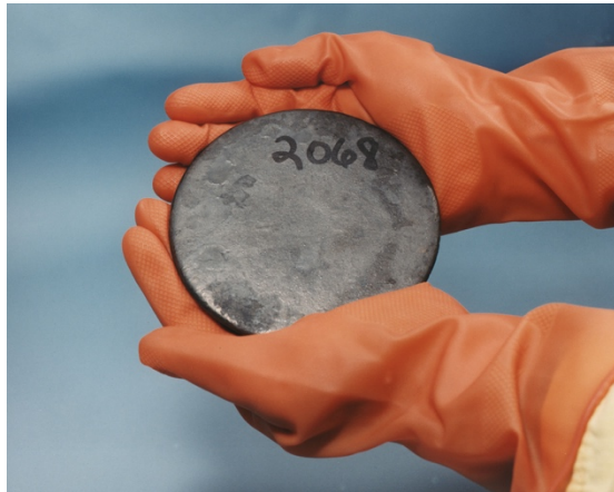
A billet or slug of enriched uranium, a fissile material, for a fuel rod in a civilian nuclear power generating reactor.
