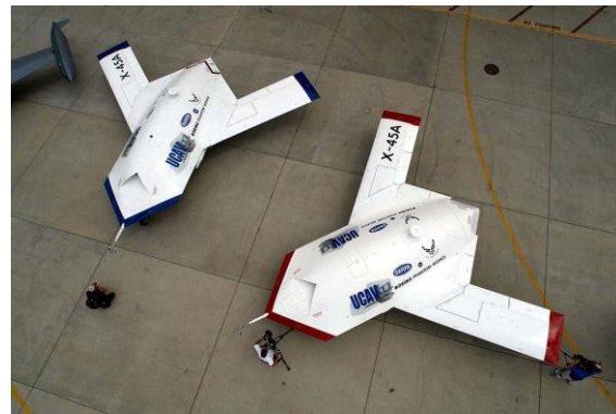
X-45A experimental U.S. unmanned combat air vehicles made by Boeing. Each X-45A is over 26 feet long, wingspan of 34 feet, and weighs 8,000 lbs empty.
