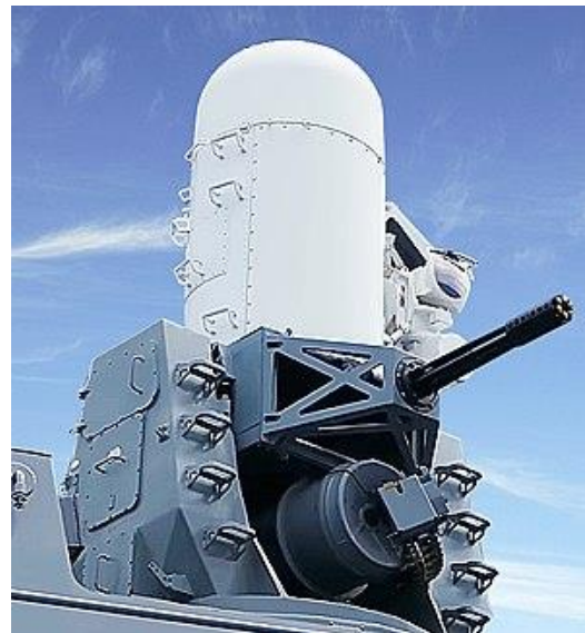
An early autonomous weapon system, the US Phalanx close-in weapon system, used mostly for defense of ships against missile attacks. First operation in 1980
