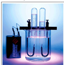
Figure 17.20: The electrolysis of water produces hydrogen gas at the cathode (on the right) and oxygen gas at the anode (on the left).
