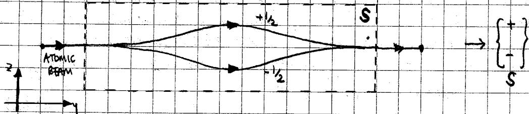
We also have the ability to insert plates to block either of the beams
