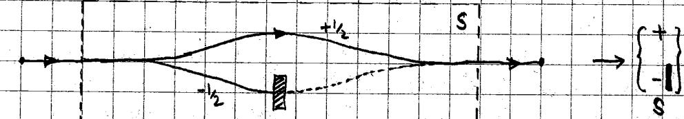
If we then put a second S-apparatus, identical to the first after it, the beam would only follow the upper path. Thus our apparatus, complete with blocking plates can act as a filter.
