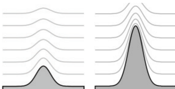
Diffusion Instability. Bumps attract diffusing particles, which follow the gradient of a certain potential field. As it grows, the gradient increases, so a bump grows unstably.
