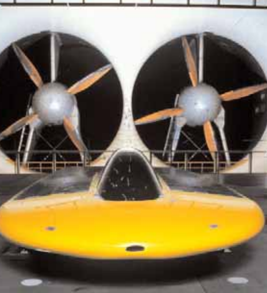
The University of Michigan solar-powered car is tested in the Langley Full-Scale Tunnel prior to entry in SunRayce '97. The tests concentrated on reducing the drag of the vehicle. Photo courtesy of NASA.
